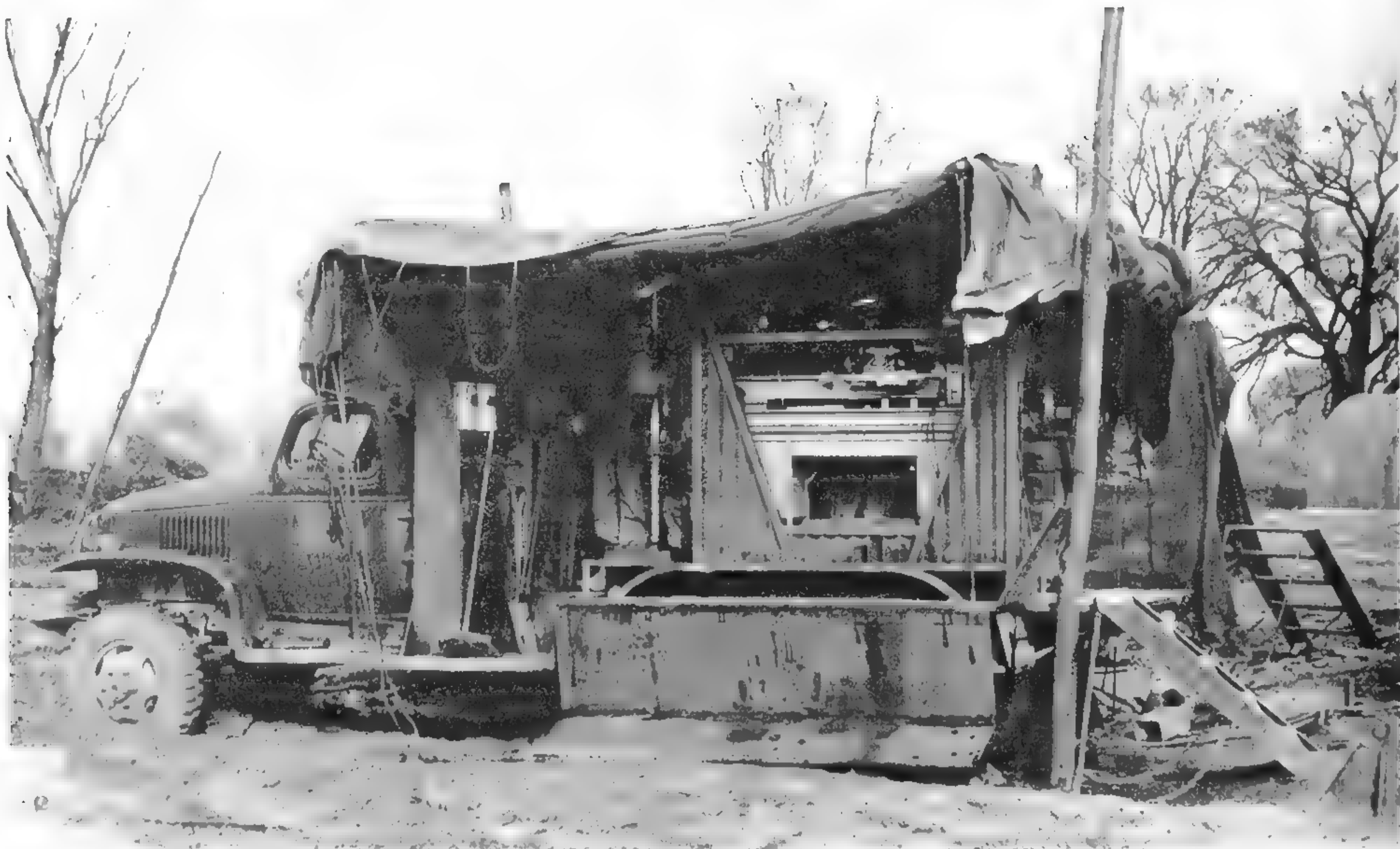
The engineer-type bodies had sides that opened up, with the lower portion hanging down to form walkways, and the upper portion hinging to form awnings. (Photo courtesy of United States Army Engineer School History Office)
